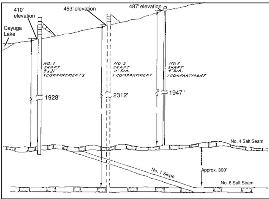
**CROSS SECTION** - When Cayuga Rock salt began mining operations in July 1920, extraction took place at the 1400 foot level. By the time Cargill purchased the mine in 1969, all activity was at the 1900 foot No. 4 level salt seam. Cargill developed the No. 6 salt seam approximately 2300 feet beneath the surface where it mines and screens rock salt before sending it to the surface for bulk loading and packaging as Halite..
